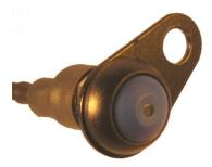
The Switch Mounting Plate is attached to either left or right Handlebar Switch Clamp. Remove the lower screw and reattach with the plate underneath the screw. Ensure the loom is routed so that it is not stretched or snagged as the 'bars are moved from lock to lock.
